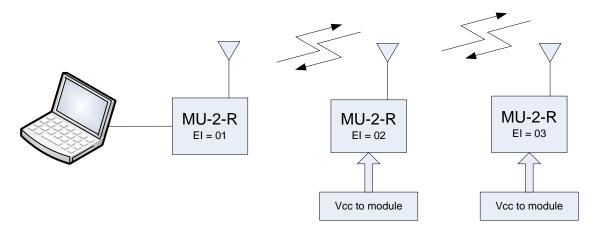
Open evaluation software and set the **Source EI = 01**, **Relay EI = 02**, **Target = 03**. Enter command "@CP03ABC/02,03" in the source window.
