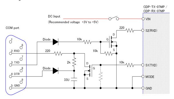
For the FETs, general switching FETs (N-ch) operating at low voltage can be used. Transistors (NPN) are also usable.
