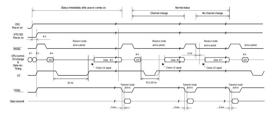
Figure 3: Timing diagram for STD-302
