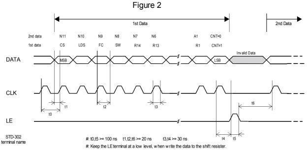
The PLL IC, which operates as shown in the block diagram in the manual, shifts the data to the 19-bit shift register and then transfers it to the respective latch (counter, register) by judging the CNT control bit value input at the end.
